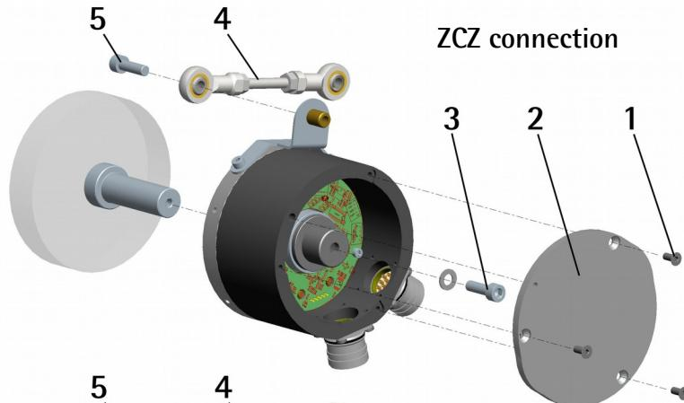
Radial runout must not exceed 0.1 mm
