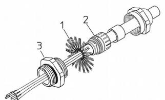
Disentangle and shorten the shielding **1** and then bend it over the part **2**; place the ring nut **3** of the connector. Be sure that the shielding **1** is in tight contact with the ring nut **3**. Do not connect unused signals.
